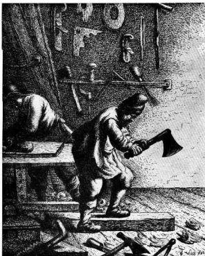
Figure 28.—About 1631: The preceding illustrations emphasize the divergent appearance of European and Anglo-American tools. This, however, was not always the case. The woodworker's shop by the Dutch engraver Jan Van Vliet suggests the similarity between English and European tool types in the 17th century. Note in particular the planes, axe, brace, and auger as compared to Moxon. (Library of Congress, Division of Prints and Photographs.)
