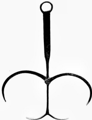
Figure 20.—Early 19th century: The double calipers of the woodturner permitted double readings to be taken without changing the set of the tool. Inherent in this practical design is a gracefulness of line seldom surpassed. (Private collection. Smithsonian photo 49793-C.)
