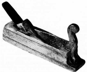
Figure 23.—1809: This bench plane of German origin is dated 1809. It is of a traditional form that persists to the present day. The planes pictured in figures 21, 22, and 23 are similar to the type brought to North America by non-English colonists. (Private collection. Smithsonian photo 49793-F.)
