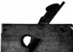
Figure 25. 1830–1840: The design of the rabbet plane, used to cut a groove of fixed width and depth on the edge of a board, was not improved upon in the 19th century. The carpenter's dependence on this tool lessened only after the perfection of multipurpose metallic planes that could be readily converted to cut a "rabbet." (Private collection. Smithsonian photo 494789-H.)
