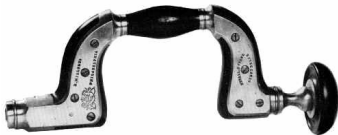
Figure 57.—1876: Jappaned and splinted with heavy brass, this brace was among the award-winning tools exhibited at the Centennial by E. Mills and Company of Philadelphia. (Smithsonian photo 49792-D.)
