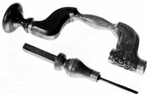
Figure 39.—18th century: The transitional form of the wooden brace and bit incorporated the overall shape of the mass-produced version but retained the archaic method of fastening the bit to the chuck. The tool is of Dutch origin and suggests the influence of Sheffield design on European tools. (Smithsonian photo 49792-E.)
