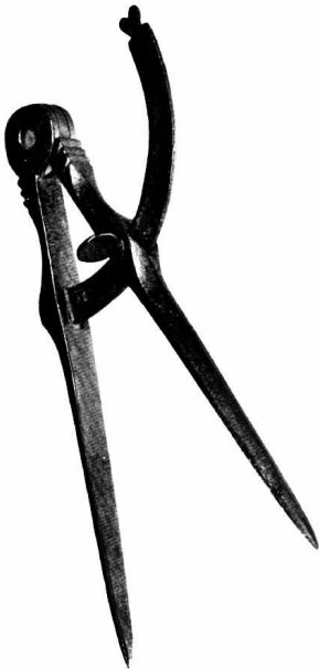
Figure 15.—18th century: Cabinetmaker's dividers of English origin. (Private collection. Smithsonian photo 49789-B.)
