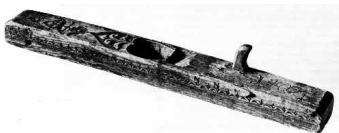
Figure 21.—1704: The floor plane or long joiner of Norwegian origin exhibits the characteristic decoration of the stock and mouth, patterns common on tools of northern European and Scandinavian origin. (Courtesy of the Norsk Folkemuseum, Oslo, Norway.)
