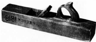
Figure 26.—1818: The jack plane, used first by the carpenter for rapid surfacing, is distinguished primarily by the beveled and slightly convex edge of its cutting iron. As with the plow and the rabbet, its shape is ubiquitous. Dated and marked A. Klock, this American example follows precisely those detailed in Sheffield pattern books. (Smithsonian photo 49794-C.)
