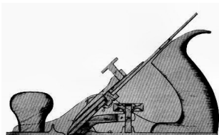
Figure 64.—1867: The drawing accompanying B.A. Blandin's specification for an "Improvement in Bench Planes" retained only the familiarly shaped handle or tote of the traditional wood-bodied plane. This new shape rapidly became the standard form of the tool with later variations chiefly related to the adjustability of the plane-iron and sole. (Wash drawing from U.S. Patent Office, May 7, 1867, Record Group 241, the National Archives.)
